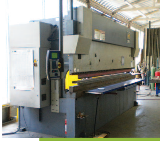
The 14-ft., 200-ton Haco-Atlantic Synchronmaster allows Phoenix Metalworks to bend 12-ft. pieces of material in a continuous mode.
